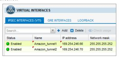
In the IPsec VPN module (VPN section), under the Site to site (gateway-gateway) tab, you will be able to define the tunnels below using the following objects:
