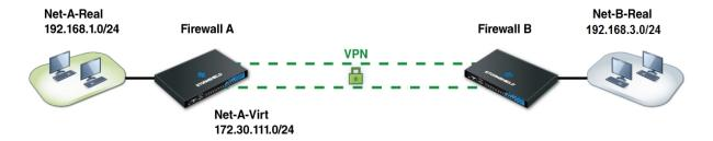
In this example, Net-A-Real located behind Firewall A will appear as Net-A-Virt to site B.
