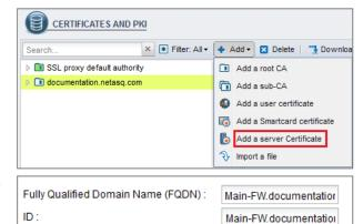
Fill in the field **Fully qualified domain name** with the FQDN of the main IPS-Firewall.
