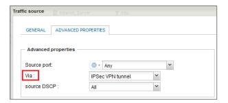
In the case presented, a client workstation located on the local network of the **remote site** must be able to connect in HTTP to the intranet server located on the local network of the **main site** (rule no. 1). You can also temporarily add, for example, ICMP to test the setup of the tunnel more easily (rule no. 2).
