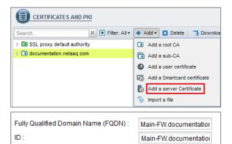
Fill in the field **Fully qualified domain name** with the FQDN of the main IPS-Firewall.
