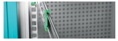
Push the chassis into the rack until both rails snap in.
