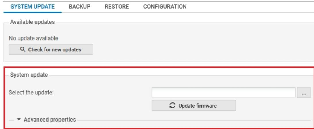
3. The update will start: **do not unplug the firewall during the operation**. The firewall will restart when the update is complete.
