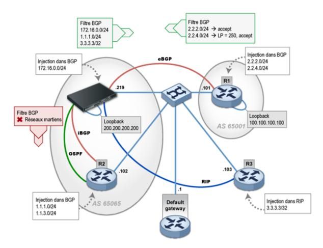
The client's network includes routers R2, R3 and the Stormshield Network firewall. Router R1 is an external BGP neighbor. This network represents a realistic architecture setup, except for the fact that all routers are physically connected through a single LAN.
