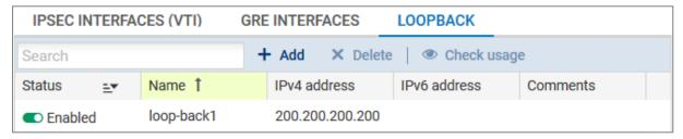
It is advisable to declare the static route to the remote loopback on the firewall outside the Bird configuration via the **Routing** module in the *Static routes* tab, in order to prevent BGP traffic from being blocked by "IP address spoofing" alarms:
