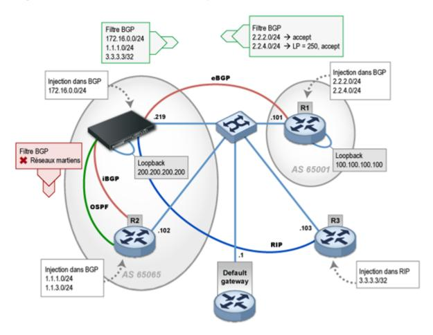
The client's network consists of the router R2, R3 and Stormshield Network firewall. The router R1 is an external BGP neighbor. This network represents a realistic architecture model, except for the fact that all the routers are physically connected by a single LAN.
