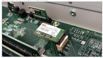
4. To extract the flash module, pull it gently and perpendicular to the motherboard:
