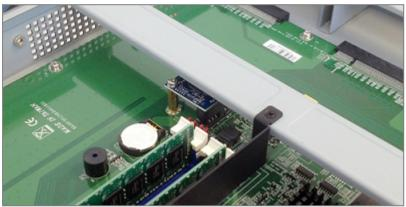
4. Unscrew the fastening screw of the Flash module with a Philips screwdriver, by keeping the associated hex spacer in place with a flat wrench:
